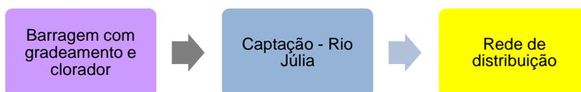
FIGURA 234 – FLUXOGRAMA DO SUBSISTEMA JÚLIA – SISTEMA CENTRO
