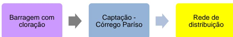
FIGURA 308 – FLUXOGRAMA DO SUBSISTEMA 02 – SISTEMA PARAÍSO
