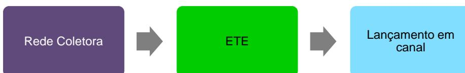
FIGURA 436 – FLUXOGRAMA DO SES FRADE – SUBSISTEMA 01
