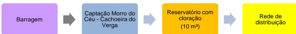
FIGURA 375 – FLUXOGRAMA DO SUBSISTEMA MORRO DO CÉU – SISTEMA PROVETÁ
