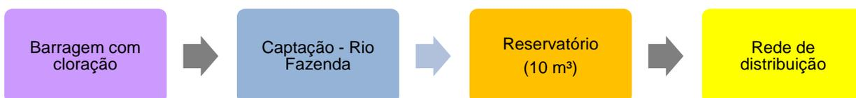
FIGURA 337 – FLUXOGRAMA DO SISTEMA SACO DO CÉU
