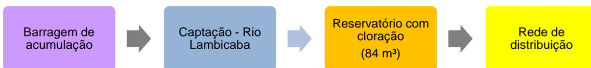
FIGURA 292 – FLUXOGRAMA DO SISTEMA LAMBICADA
