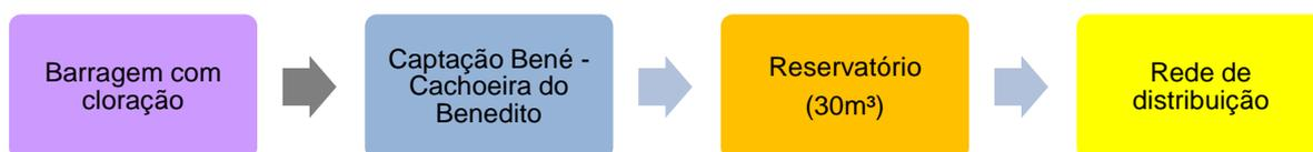
FIGURA 357 – FLUXOGRAMA DO SUBSISTEMA BENÉ – SISTEMA ARAÇATIBA
