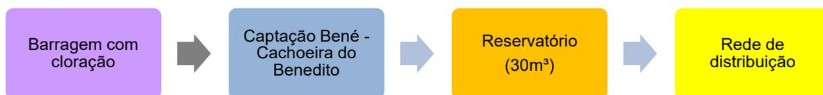
FIGURA 5-148 – FLUXOGRAMA DO SUBSISTEMA BENÉ – SISTEMA ARAÇATIBA
