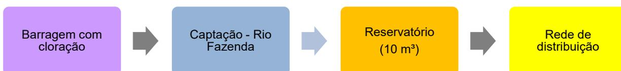
FIGURA 5-134 – FLUXOGRAMA DO SISTEMA SACO DO CÉU
