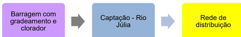
FIGURA 5-82 – FLUXOGRAMA DO SUBSISTEMA JÚLIA – SISTEMA CENTRO
